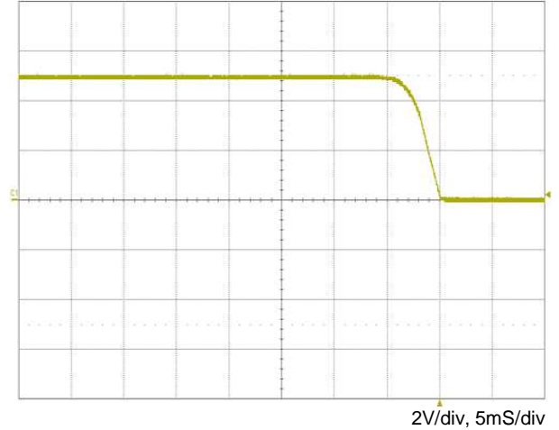
Output turn-off rated load
